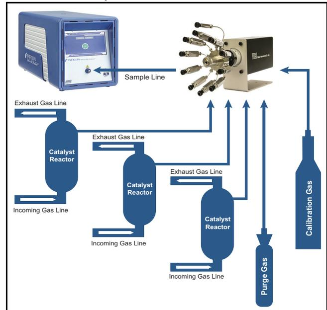
Among the selector models, SD and SF selectors suit most application needs. The SD selector is dead-ended, allowing the user to conserve valuable samples; whereas, the SF selector has a flow-through configuration, allowing fresh samples to pass through each valve continuously. (See Figure 2.)
