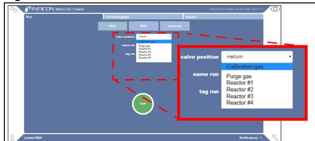
The Valco Configuration screen enables users to name each sample port position on the Valco stream selector. (See Figure 6.)
