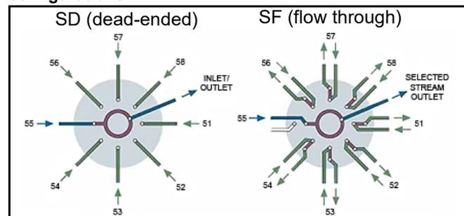
INFICON offers a 10-port SD (dead-ended) and a 10-port SF (flow-through) Valco stream selector accessory package pre-assembled from the factory. The pre-assembled Valco stream selectors have 1/16 in. sample line filters installed and leak checked at each inlet port. (See Figure 3.) Simply connect the sample lines and the Valco stream selector is ready to use.
