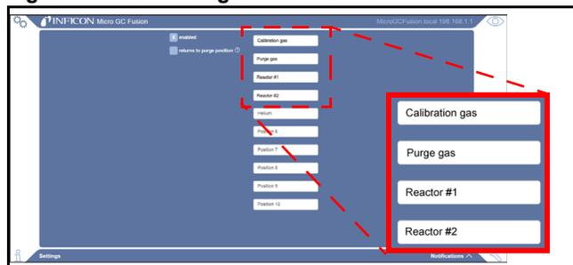
The user defined sample port names are selectable on the main screen and the Sequence Editor screen. (See Figure 7.)
